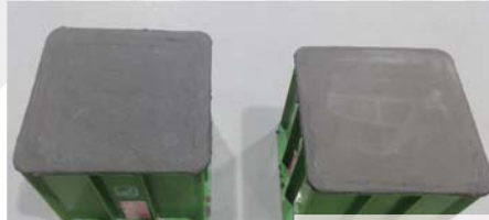
Without CCP Primer With CCP Primer put into oven at 75°C for 48 hours
