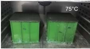
After CCP Primer was dry (~12hrs), put the specimens with/without CCP in the oven 75°C for 48 hours.
