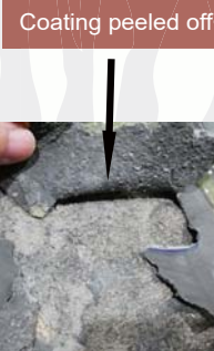
Without CCP Primer With CCP Primer put into oven at 75°C for 48 hours
